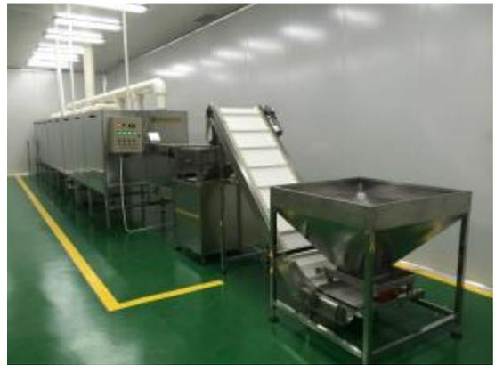
50kw Microwave baking equipment/Customized microwave baking equipment
